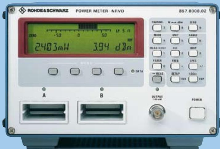
The R&S® NRVD covers a total bandwidth of 40 GHz and a power span from 100 pW up to the kW range. Being individually and absolutely calibrated, the sensors can be interchanged as required without impairing measurement accuracy.
