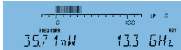
*Readout of pulse power after entry of duty factor*
