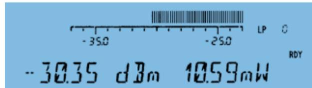
*Readout of correction frequency together with measured value*
