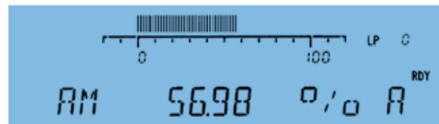
*Readout of reflection coefficient*
